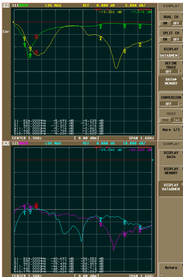
Figure 41 and 42: |S_{11}| and |S_{21}| comparison between a 900 MHz tuned half wavelength dipole and a penta-band internal antenna, if |S_{21}| like in marker 3 area are similar the target antenna performances are good
